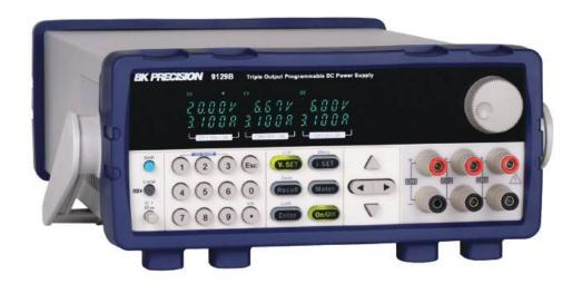
The 9129B is an economical triple output linear programmable DC power supply featuring isolated outputs that can be adjusted independently or combined in series or parallel to output higher voltage or current. Additionally, this supply can operate in tracking mode with user-configurable ratios between channels.
